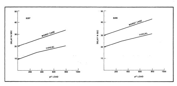
Figure 5. Output Delay vs. Capacitance
